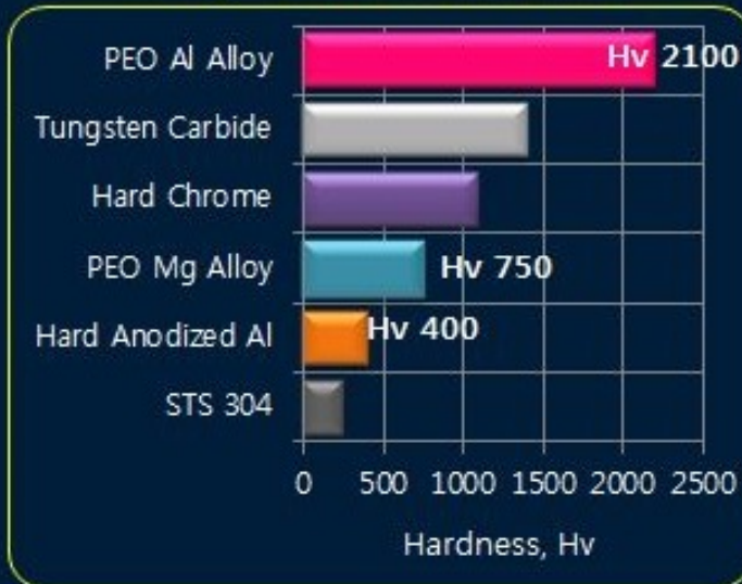
Comparative Hardness (HV)
