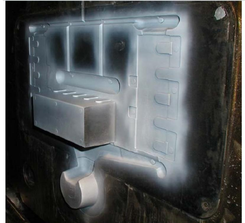
Aluminium die casting mould with BN release coating
