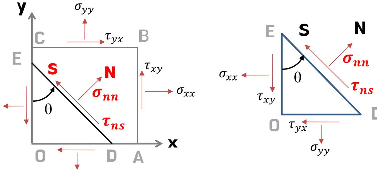
$$\sigma_{nn} \cdot (\overline{DE}) = \sigma_{xx} \cos\theta \cdot (\overline{EO}) + \tau_{xy} \sin\theta \cdot (\overline{EO}) + \sigma_{yy} \sin\theta \cdot (\overline{OD}) + \tau_{yx} \cos\theta \cdot (\overline{OD})$$
