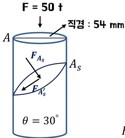
$$F = 50 \text{ t} = 50,000 \text{ kg} = 490,500 \text{ N} \quad 1 \text{ kg} = 9.81 \text{ N}$$
