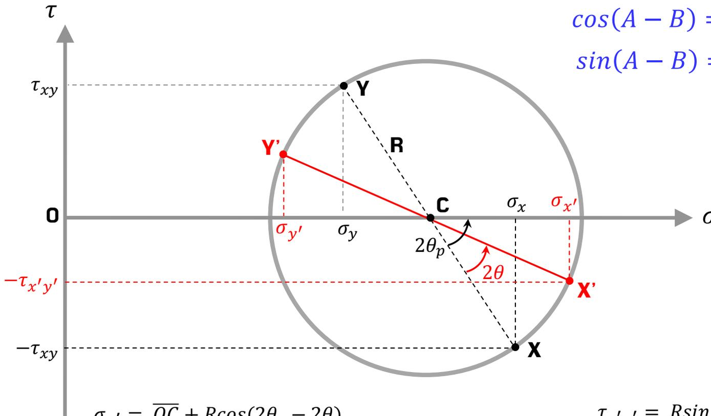
$$\begin{aligned} \sigma_{x'} &= \overline{OC} + R \cos(2\theta_p - 2\theta) \\ &= \frac{\sigma_x + \sigma_y}{2} + R(\cos 2\theta_p \cos 2\theta + \sin 2\theta_p \sin 2\theta) \\ &= \frac{\sigma_x + \sigma_y}{2} + R \left( \frac{\sigma_x - \sigma_y}{2} \cdot \cos 2\theta + \frac{\tau_{xy}}{R} \cdot \sin 2\theta \right) \\ &= \frac{\sigma_x + \sigma_y}{2} + \frac{\sigma_x - \sigma_y}{2} \cos 2\theta + \sin 2\theta \cdot \tau_{xy} \end{aligned}$$
