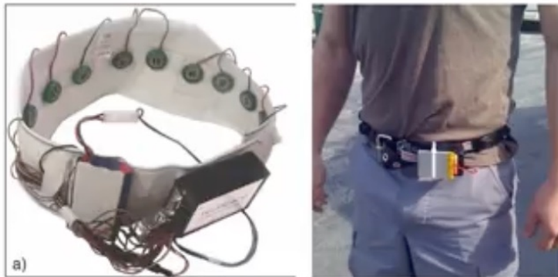
Haptic belt: Direction sense
